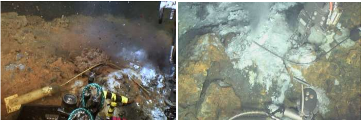
Fig. 4.8-2 MISO 102-Left shows instrument at Diva before recovery in 2017 showing the tip of the wand not in the hot fluid. Right-image of probe at deployment in 2015. Jason was positioned in opposite headings between the 2 years.
