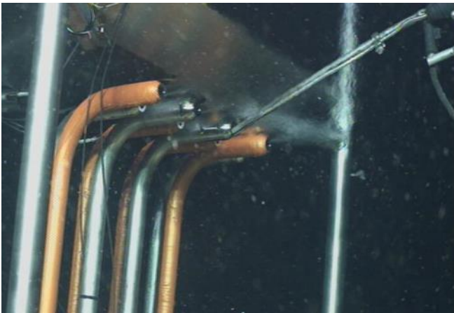
Fig. 4.6-21. Using thermal probe to determine temperature coming out of Creare tubes; max temperature of 116.4°C.
