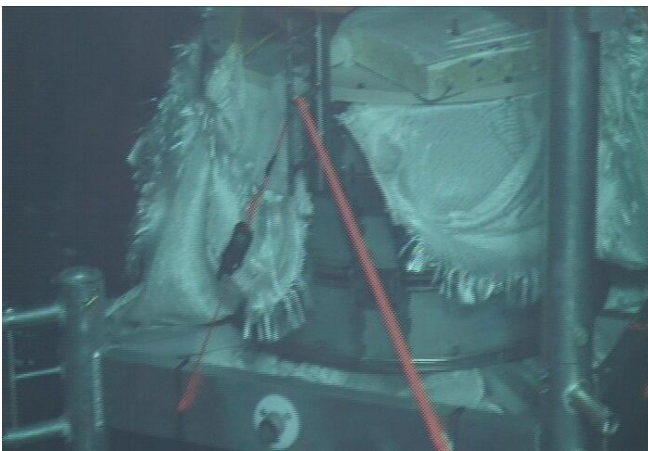
Fig. 4.6-3. Damaged skirt; device secured to elevator.
