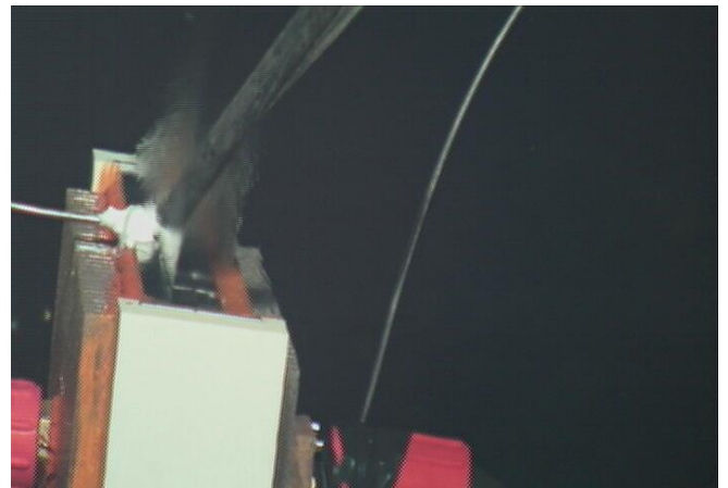
Fig. 4.6-16. Measuring temperature of effluent exiting the top of MAPC device; max temp of 97.8°C.
